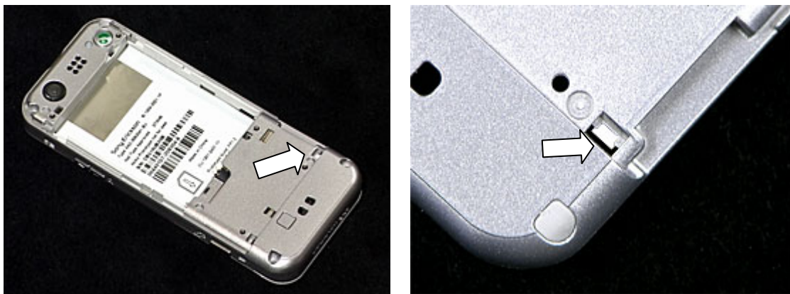
Location of the Liquid Intrusion Indicator.
